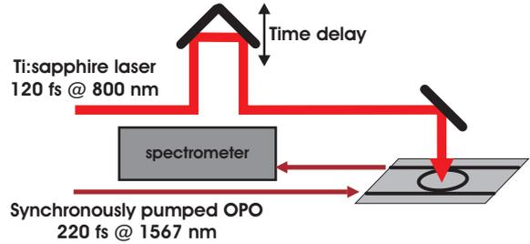
**Fig. 2:** Schematic illustration of the experimental setup for the time-resolved investigation of the switching process.
