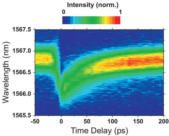
**Fig. 3:** Spectral response (intensity plot) of the implanted microring resonator measured at the drop channel after optical excitation.
