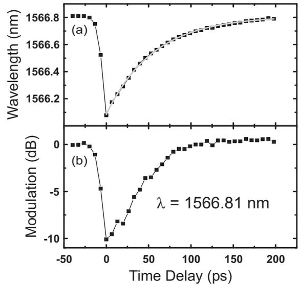
**Fig. 4:** (a) Time resolved shift of the peak resonance wavelength at the drop waveguide (squares). The grey solid line is an exponential fit to the data for positive time delays. (b) Normalized drop waveguide intensity at the resonance wavelength  $\lambda = 1566.81\ \text{nm}$ .
