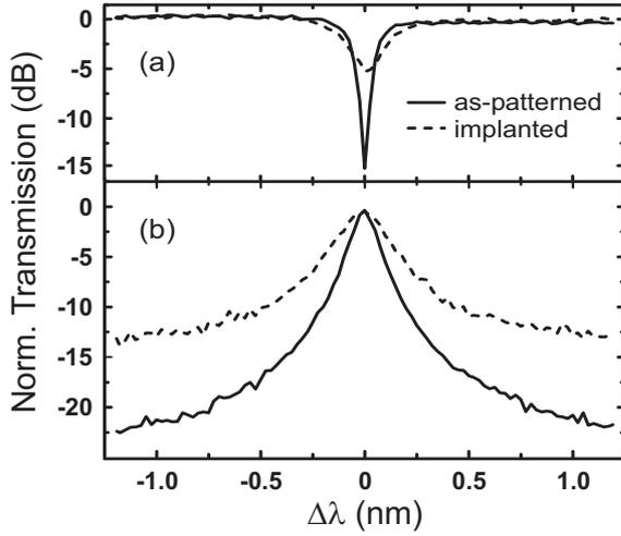
**Fig. 1:** Transfer function of the investigated microring resonator after EBL patterning (solid lines) and after additional  $O^+$  ion implantation at energy of 120 keV and dose of  $1 \times 10^{12} \text{ cm}^{-2}$  (dotted lines). (a) drop port and (b) through port.  $\Delta\lambda = \lambda - \lambda_0$ , with  $\lambda_0$  the resonance wavelength.
