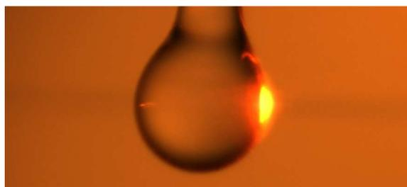
**Fig. 1:** Signature of fundamental WGM excitation. As the pump tapered fiber (shadow in the background) touches the sphere, an intense field is suddenly radiated at the rim of the sphere. Sphere diameter: 113  $\mu\text{m}$ ; wavelength: 0.8  $\mu\text{m}$ .
