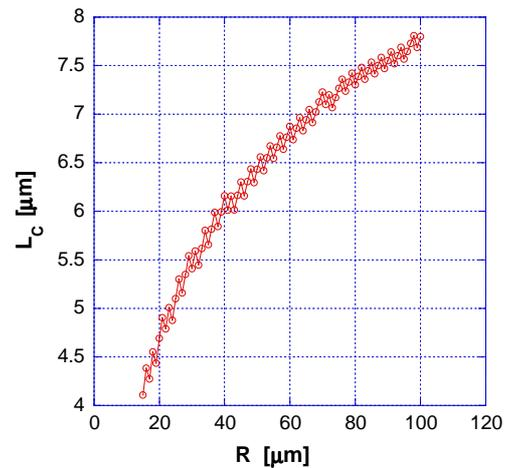
**Fig. 3:** Coherent Length ( $L_C$ ) for Second Harmonic Generation as function of the radius ( $R$ ) of sphere.
