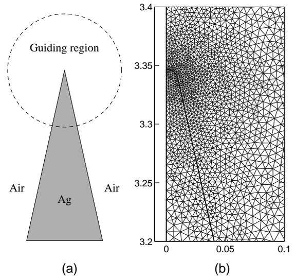
**Fig. 1:** (a) Schematic diagram of a metal wedge plasmon polariton waveguide. (b) Finite-element mesh of a metal wedge guide with  $\Lambda$  angle at 25 degree. Only half of the waveguide is used by using perfect magnetic conductor (PMC) condition at its symmetry line ( $x = 0$ ). The tip is rounded with an arc with 10nm radius. Axis unit:  $\mu\text{m}$ .
