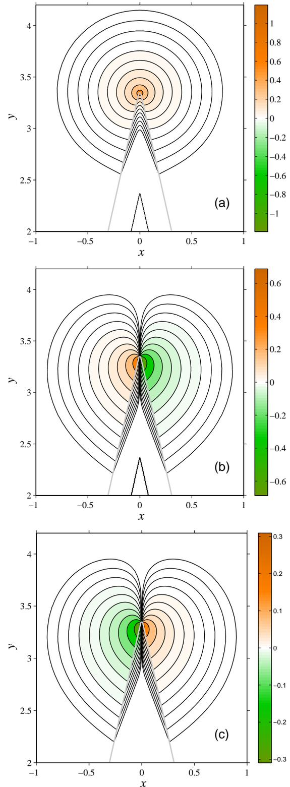
**Fig. 3:** (Color online) H field components of a mode guided by a wedge with a  $25^\circ$  angle. (a)  $H_x$  component; (b)  $H_y$  component; (c)  $H_z$  component. Orange for positive, and green for negative. Contour lines (except the first one, which is at 90% of the maximum value) are in 3dB separation. The void regions within the metal wedge as appeared in (a) and (b) are not computed as the field there can be safely treated as zero.
