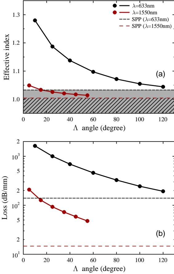
**Fig. 2:** (Color online) Dispersion (a) and loss (b) curves of the guided WPP mode as  $\Lambda$  angle changes. Gray (line-shaded) region in (a) is the allowed states by an Ag-air interface at  $\lambda = 633\text{nm}$  ( $1550\text{nm}$ ).
