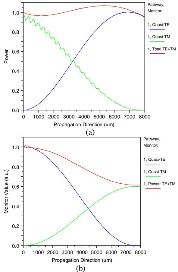
**Fig. 4.** 3D BPM simulation of polarisation conversion in anisotropic channel waveguide directed at angle  $q=5.7^\circ$ . Input polarisations: (a) TM (b) TE.
