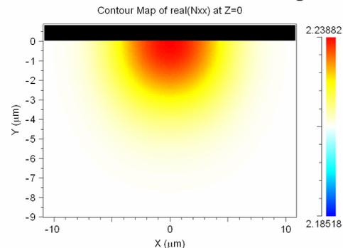
**Fig. 1.** Simulated distribution of refractive index in channel waveguide.  $w=8 \mu\text{m}$ ,  $h=3.5 \mu\text{m}$ ,  $dN=0.03$ .
