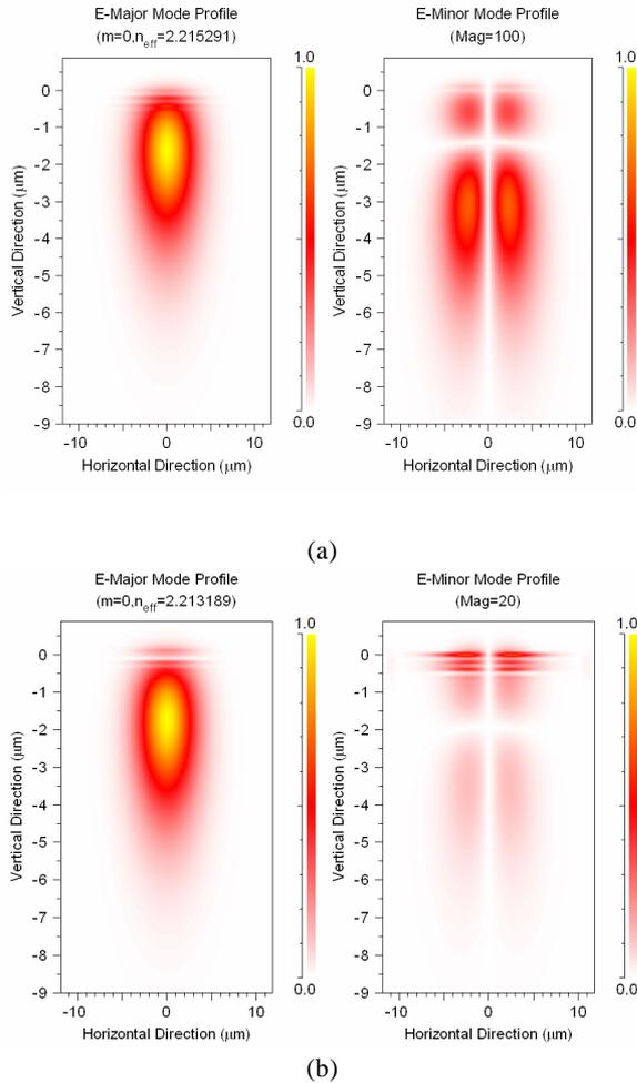
**Fig. 2.** Simulated distribution of optical filed of guided modes in diffused waveguide presented in Fig. 1. (a) quasi-TE mode, (b) quasi-TM mode.  $q=0$ .
