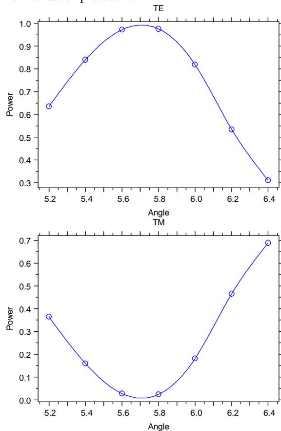
**Fig. 5.** 3D BPM simulation of polarisation conversion at different angle  $q$  relative to  $X$ -axis in  $Y$ -cut  $Ti:LiNbO_3$ . Input polarisations: (a) TM (b) TE.
