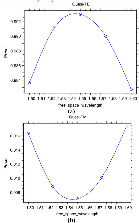
**Fig. 6.** 3D BPM simulation of polarisation conversion at different optical wavelengths in anisotropic channel waveguide directed at angle  $q = 5.7^\circ$ . Input polarisations: (a) TM (b) TE.
