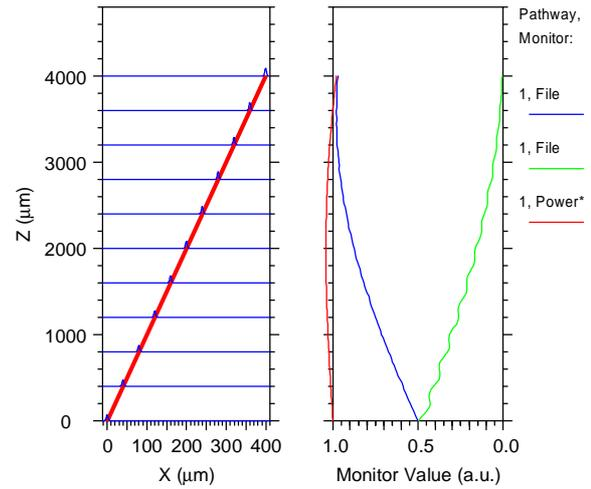
**Fig. 3.** 3D BPM simulation of polarisation conversion in anisotropic channel waveguide directed at angle  $q=5.7^\circ$ . Input polarisations: TE&TM.
