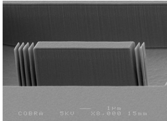
Fig. 3: 6  $\mu\text{m}$  deep DBR gratings in InP
