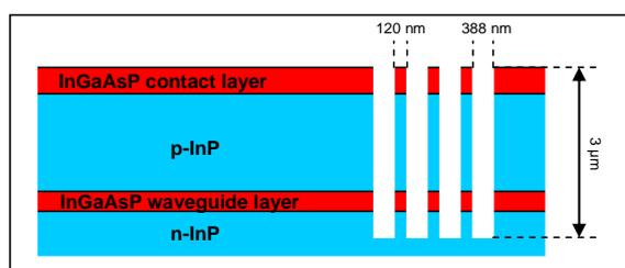
Fig. 1: Schematic drawing of deep-etched DBR grating
