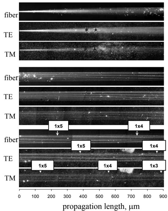
Fig.4 The successive sequences of recorded mode field interference images for MMI section of the width 60 $\mu\text{m}$ , excited at 1/3<sup>rd</sup> of the section width.
