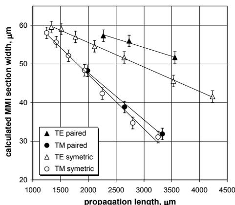
**Fig.7** The dependence of calculated MMI section width on the propagation length for MMI section of the width  $60\ \mu m$ .
