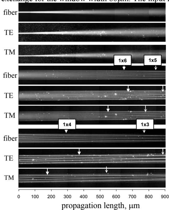
Fig.3 The successive sequences of recorded mode field interference images for MMI section of the width 60 $\mu\text{m}$  symmetrically excited (a)
