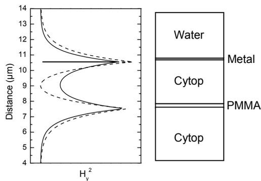
**Fig. 3:** Vertical mode profiles (solid line: symmetric, dashed line: antisymmetric) of a structure shown on the right, consisting of a 49 nm PMMA “feeding core,” a 3.0  $\mu\text{m}$  intermediate cladding layer and an 8 nm gold film surface waveguide.
