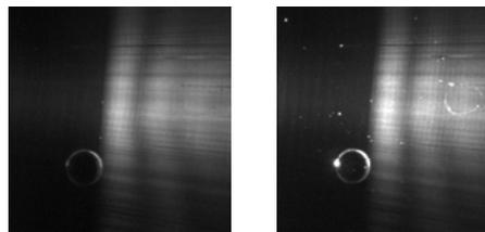
**Fig. 4:** Fluorescence induced on a waveguide chip with a metallic surface waveguide covering the chip in the right half of the images, with (left image) and without (right image) filtering of the excitation wavelength. The images are 1 mm across and light is incident from the left side.
