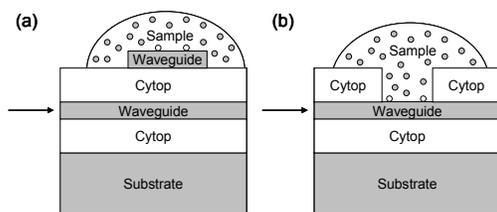
**Fig. 1:** Waveguide configurations used in the present study. (a) Coupled-waveguide structure using a buried “feeding core” waveguide and a surface “sensing” waveguide. (b) Single-waveguide structure with a sample well exposing part of the waveguide. Samples consisted of fluorescent beads in solution. Fluorescence is excited at the waveguide surface as indicated by the white beads.
