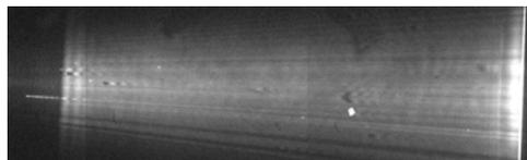
**Fig. 5:** Fluorescence excitation over a 5-mm wide gold film. The propagating mode is confined mainly to the dielectric feeding core. Initial beating with the rapidly decaying mode confined mainly to the metal film can be observed at the left side of the film.
