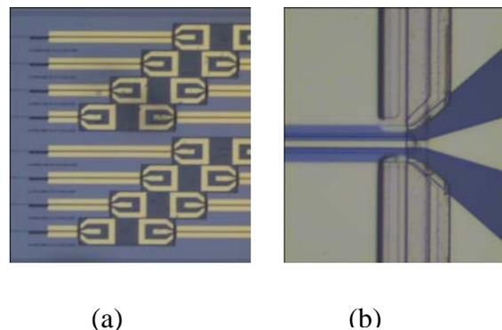
**Fig. 3:** Integrated circuits after complete fabrication are shown, from left to right 3  $\mu\text{m}$  input waveguide of 500  $\mu\text{m}$  length, converter section of 150  $\mu\text{m}$  length, then detectors with varying lengths (a), the edge of the detector is shown in (b).
