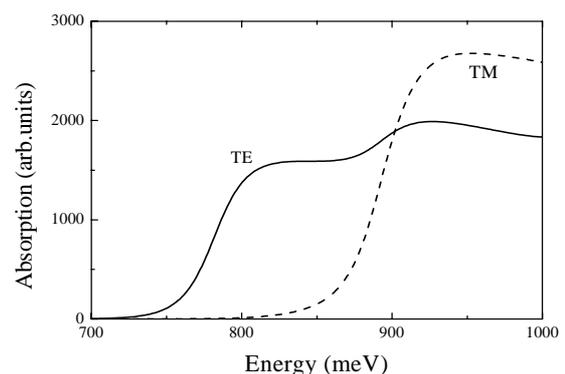
**Fig. 1:** Calculated absorption spectrum of a 4 nm compressively strained In<sub>65</sub>Ga<sub>35</sub>As quantum well with InGaAsP barriers
