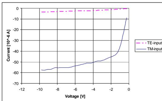
**Fig. 5:** Experimental results for the integrated waveguide-detector. Top: IV-curve of a 1 mm long detector with -6.1 dBm input power in TE and TM polarization. Bottom: Responsivity as a function of detector length, for TM polarized input power
