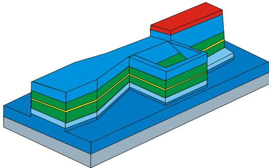
**Fig. 2:** Integrated waveguide and detector within POLIS (before metal contacts are applied). From left to right the input waveguide, a taper, the polarization converter (with the sloped side inside a wall that defines the wet etch region) and the detector are shown.
