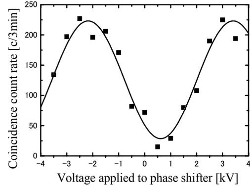
Fig. 6: Experimentally observed photon intensity interference.
