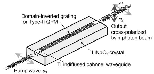
**Fig. 1:** Configuration of Type-II QPM waveguide NLO cross-polarized twin photon generation device.
