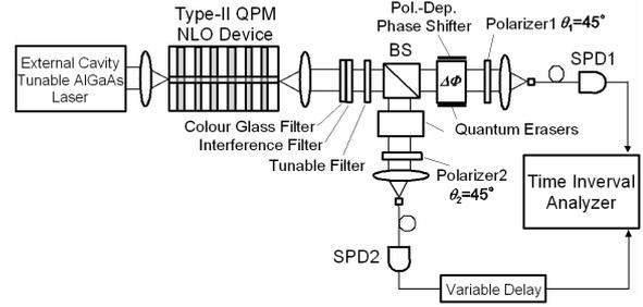
Fig. 5: Setup for polarization entangled state generation and measurement.
