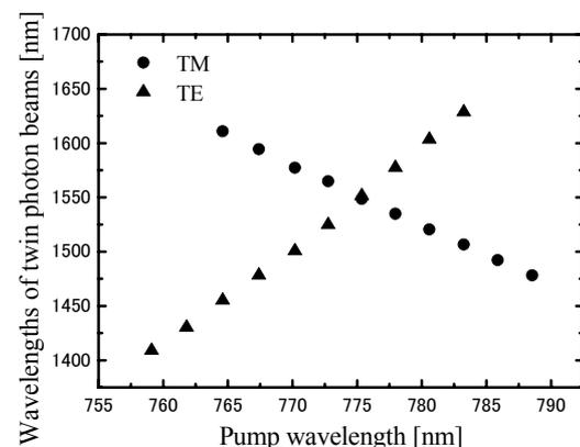
**Fig. 2:** Measured dependence of the twin-photon wavelengths on the pump wavelength.
