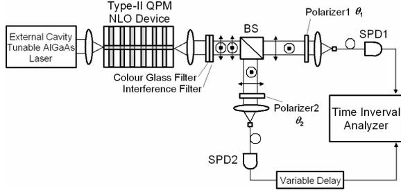
Fig. 7: Setup for twin photon polarization measurement.
