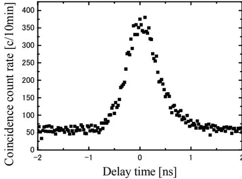
**Fig. 4:** Correlation of the cross-polarized twin photons.
