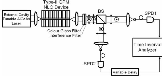
**Fig. 3:** Setup for measuring the time correlation of the cross-polarized twin photons.
