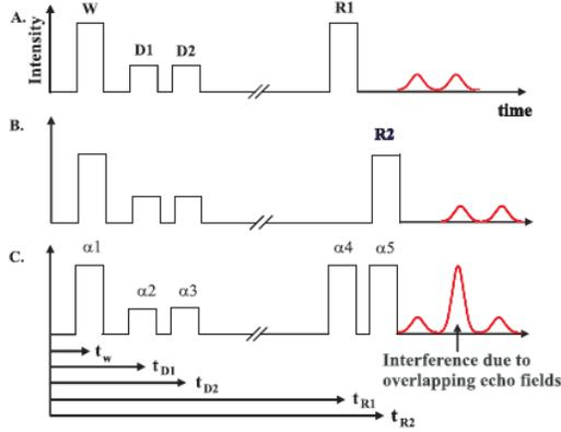
**Fig. 1:** Illustration of the sequence of pulses for the interference of photon echoes. The data is read out twice and the phase between the data (or read) pulses is changed to produce interference in the central time bin.
