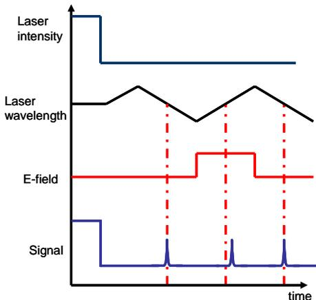
**Fig. 5:** Measurement sequence to assess magnitude and reversibility of the dc Stark shift.
