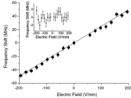
**Fig. 6:** Shift (and return) of the spectral hole's central frequency as a function of the electric field in the Erbium doped  $\text{LiNbO}_3$  waveguide.
