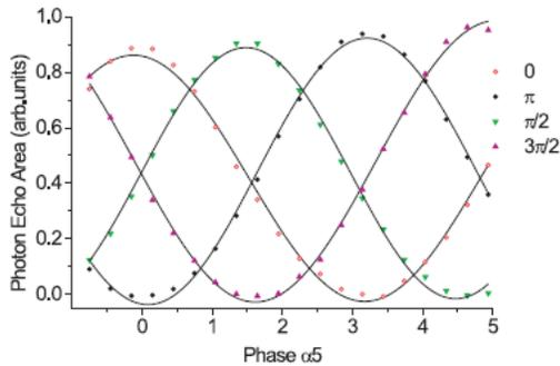
**Fig. 3:** Area under the central echo as function of the phase of the second read pulse. All four classical states, analogous to the quantum states used in the four-state quantum cryptography protocol, are stored, retrieved and analyzed with close to 100% fidelity.
