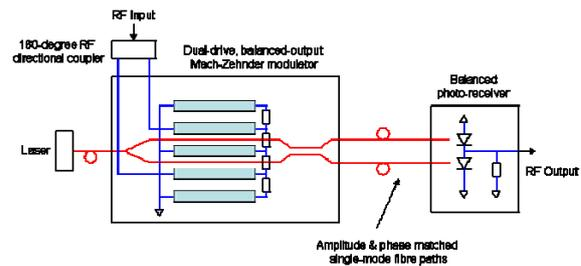
**Fig. 8:** Analogue optical link employing dual-drive Mach-Zehnder modulator and balanced photo-receiver for laser RIN suppression.
