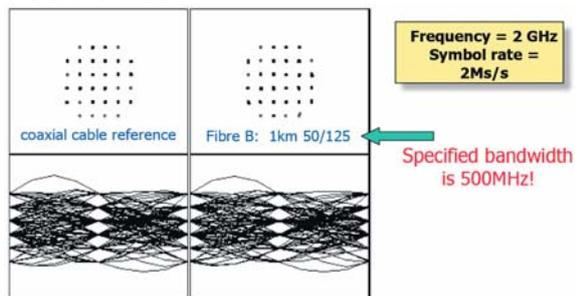
**Fig. 10:** Constellation and eye diagram for 32-QAM transmission at 2 GHz and 2 Ms/s. Left is coaxial cable (reference) and right is fibre reel B
