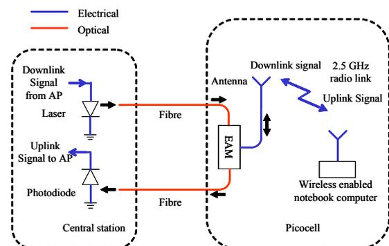
**Fig. 1:** Schematic representation of the Picocell experiment using a waveguide type EAM transceiver by Wake *et al*.
