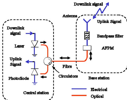
Fig. 2: A simplified wireless over fibre system concept involving an AFPM at the AU performing photo-detection for the downlink path and optical modulation for the uplink path.
