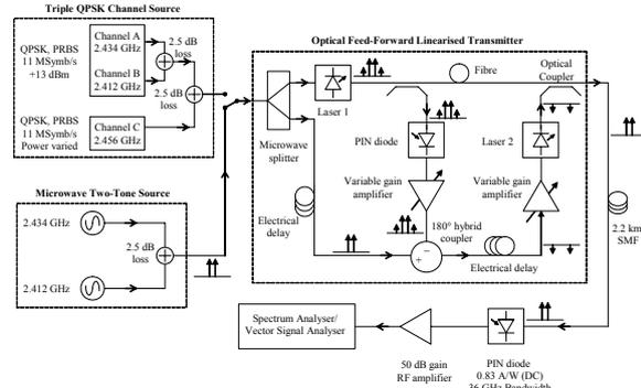
**Fig. 4:** Experimental arrangement for feed-forward linearisation and triple QPSK modulated wireless signal over fibre transmission.
