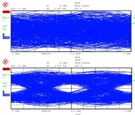
**Fig. 6:** Detected -23 dBm Channel C in-phase eye-diagrams with feed-forward disabled (upper) and enabled (lower). Channel filter bandwidth: 20 MHz.
