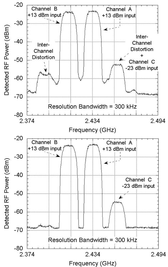
**Fig. 5:** Detected RF spectra of the three QPSK channels with feed-forward linearisation disabled (top) and enabled (bottom).
