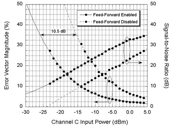
**Fig. 7:** EVM and SNR vs. Channel C input power. Channel filter bandwidth: 20 MHz.
