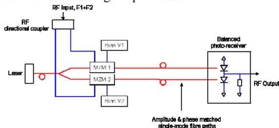
Fig. 9: Simplified experimental arrangement for the Class AB analogue optical link.
