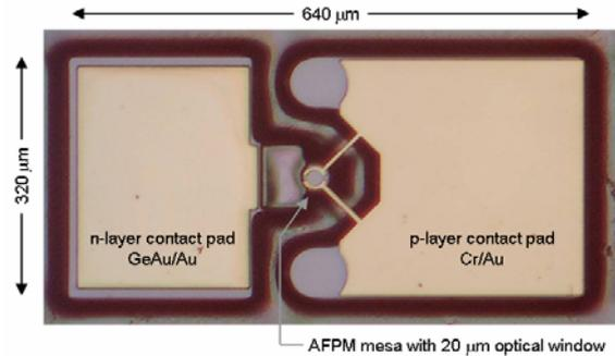
Fig. 3: Top microscopic view of a fabricated air-bridged AFPM.
