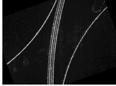
Fig. 4: Scattered light as observed from the top at 633 nm
