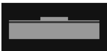
Fig. 4: Cross section of the waveguide structure used for measurements of the material losses.
