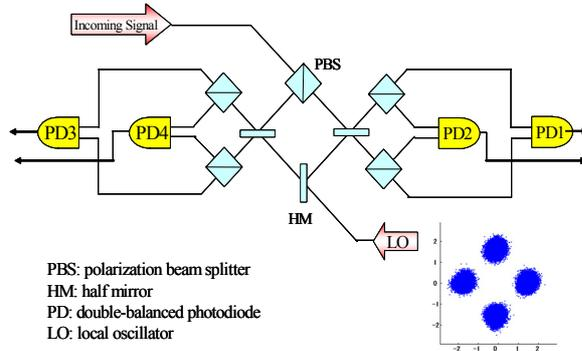
Fig. 6: Schematic diagram of the phase diversity homodyne receiver and a demodulated pattern.
