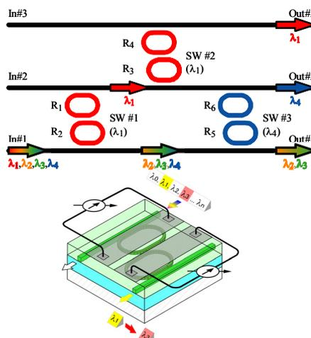
Fig. 5: Multi-port hitless wavelength selective switching circuit layout and a switching element.
