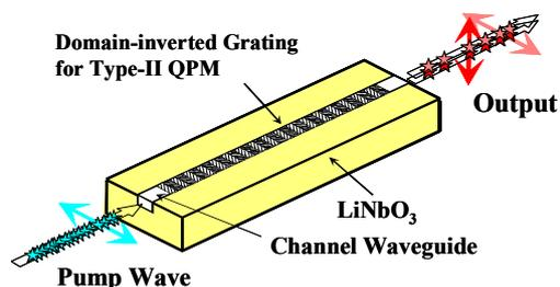
Fig. 3: Cross-polarized twin photon generation devices.
