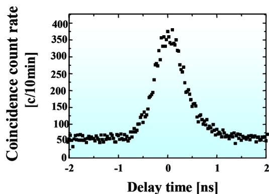
Fig. 4: Measured correlation of cross-polarized twin photons.
