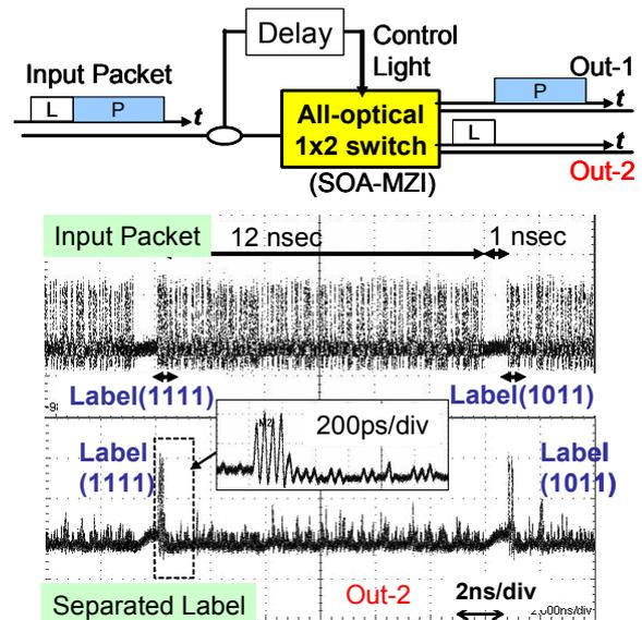
Fig. 8: Experimental result of the label separation by self-switching scheme of SOA-MZI all-optical switch.
