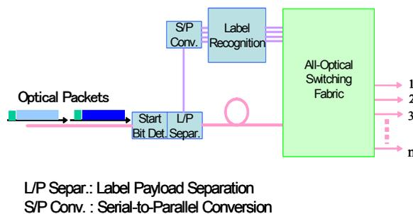
Fig. 7: Schematic diagram of the all-optical packet routing subsystem.
