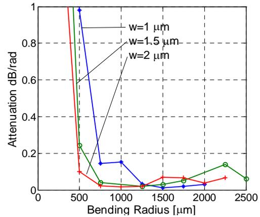
Fig. 8: Measured TE bending losses ( $t = 65$  nm).
