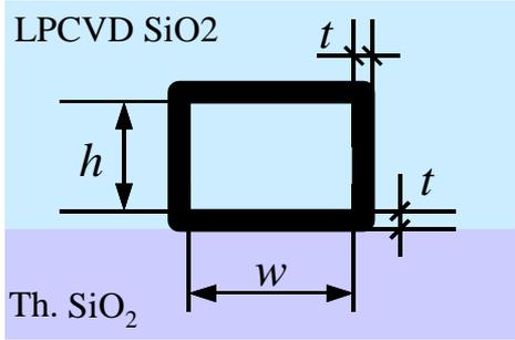
Fig. 2: Transverse shape of the realized waveguide
