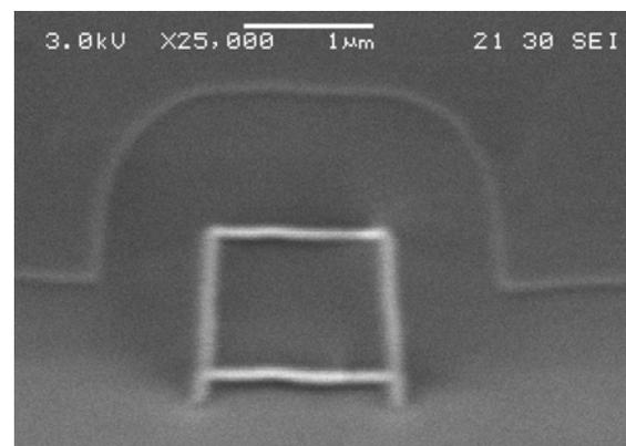
**Fig. 1:** Photograph of a box-shaped waveguide realized with TriPleX technology. The clear box is  $\text{Si}_3\text{N}_4$  65nm thick; the gray surrounding is  $\text{SiO}_2$ .
