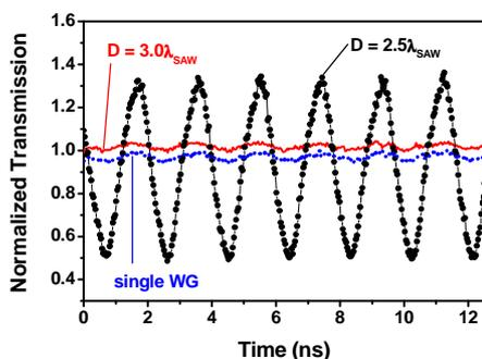
**Fig. 6:** Transmission of MZI devices with waveguide separation  $D = 3\lambda_{\text{SAW}}$  (solid line) and  $2.5\lambda_{\text{SAW}}$  (dots). The dotted line shows the transmission in a control structure where the MZI arms have been replaced by a single waveguide. All measurements were carried out by coupling an RF-power  $P_{\text{IDT}}=60$  mW to the IDTs.
