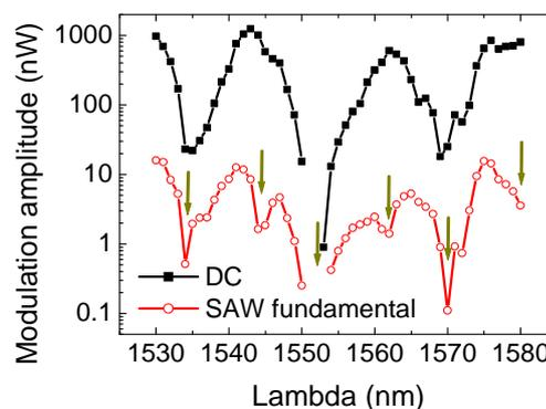
**Fig. 8:** Transmission (black line, filled symbols) and modulation (red line, open symbols) spectrum of SOI MZI with arm separation of  $D=4.5\lambda_{\text{SAW}}$ . RF power to IDTs  $P_{\text{RF}}= 50$  mW.
