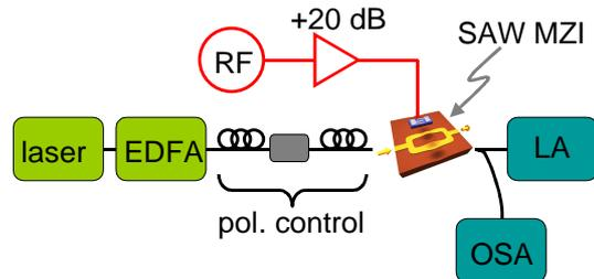
**Fig. 7:** Experimental setup for characterizing SOI modulator.
