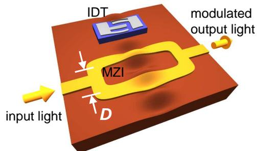
**Fig. 1:** Schematic representation of an MZI device with SAW modulation. Separation of the MZI arms,  $D$ , is an odd number of half SAW wavelengths, so that the SAW field modulates the two arms in opposite phase.
