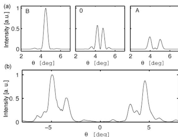
**Fig. 8:** (a) Calculated far-field line scans across the major lobes of the 3 lowest loss modes (B, 0, A) of Fig 4. (b) Measured line scan across the lower far-field lobes of Fig 7 in the coupled case.
