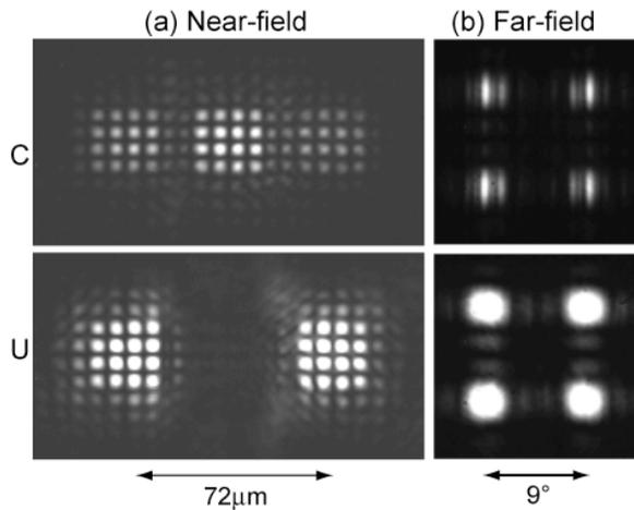
**Fig. 7:** Measured near (a) and far-field (b) patterns of coupled (C) and uncoupled (U) PhC SLs.  $I_L=690$  mA,  $I_R=700$  mA,  $I_M=0$  mA (U) and  $I_M=380$  mA (C).
