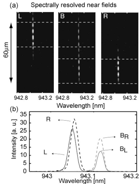
**Fig. 6:** (a) Spectrally resolved near-field of one row of the coupled PhCH islands of Fig. 5 corresponding to current injection in the left (L), right (R) and both (B) photonic island(s). (b) Line scans across the spectra (averaged between the white dashed lines) in (a). The index notation  $B_L$  and  $B_R$  relates to the spatial positions corresponding to the left and right islands, respectively.
