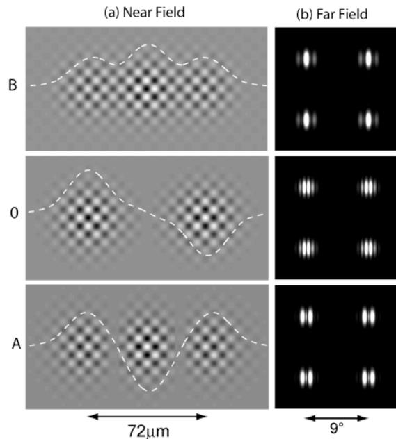
**Fig. 4:** (a) Calculated near and far-field (b) pattern of the “bonding” (B), “zeroth” (0) and “anti-bonding” (A) modes of three  $5 \times 5$  photonic island, each separated by 2 lattice periods. The dashed curve is the slowly varying envelope function along the center of the array. All other parameters are as for Fig. 2.
