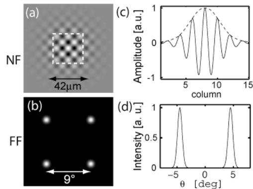
**Fig. 2:** (a) Calculated near and far-field (b) patterns of 5x5 photonic island (dashed square). (c) Near field line scan across the center of (a). (d) Far-field line scan across the main lobes.  $\lambda=940$  nm,  $\Lambda=6$   $\mu\text{m}$ , Au pixel size  $4.9\times 4.9\mu\text{m}^2$  (island),  $3\times 3\mu\text{m}^2$  (sea).
