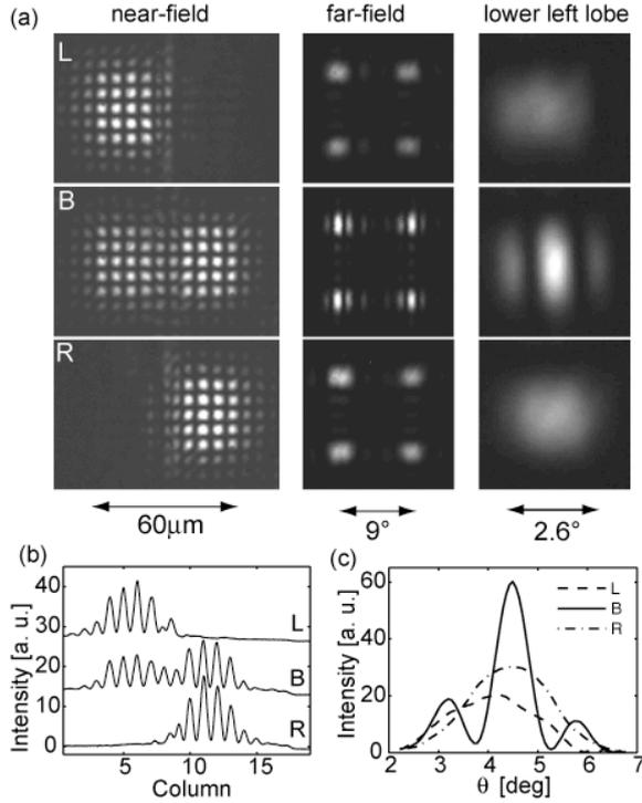
**Fig. 5:** Emission characteristics of separate-contact PhCHs incorporating two 4×5 coupled islands separated by 2 lattice periods. (a) Near-field patterns corresponding to current injection in the left (L), right (R) and both of the photonic islands (B) and corresponding far-field patterns (The light from the “sea” domain was blocked). (b) Average line scans across the near-field patterns of (a). (c) Average line scans of the lower left far-field lobes in (a).
