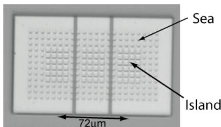
**Fig. 1:** Optical micrograph (top view) of a PhCH containing three 4x6 photonic islands defined on a VCSEL wafer.
