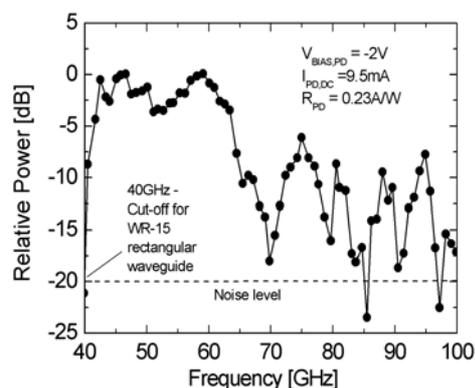
Fig. 12 Heterodyne measured AC characteristics: relative radiated RF output power vs. frequency.
