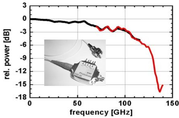
**Fig. 2:** Relative frequency response of the PD module (+2.3 dBm optical input power) measured with hp437B (black) and PM3 (red) , inset: photograph of the PD module.
