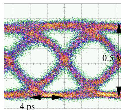
**Fig. 5** Detected eye pattern under 160 Gbit/s RZ excitation,  $V_{\text{bias}} = -2.5 \text{ V}$ .
