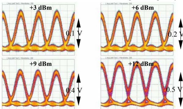
**Fig. 3** Electrical 80 Gbit/s RZ eye pattern at 3, 6, 9 and 12 dBm optical input power detected by the detector module at -2.5 V bias (x: 5ps/div).
