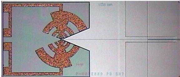
Fig. 11 Photograph of the complete photomixer chip with dimensions 2.75 x 1.4 mm<sup>2</sup>; illumination is from the right.
