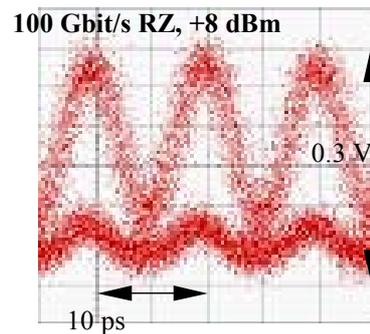
**Fig. 4** 100 Gbit/s RZ eye pattern at +8 dBm input power,  $V_{\text{bias}} = -2 \text{ V}$ ,  $2^{20}-1$  PRBS (courtesy of L. Moeller, Lucent Techn., USA).
