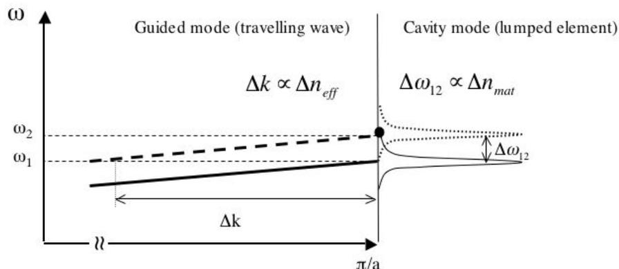
**Figure 1.** Idealised dispersion curve of a waveguide in the slow light regime. The solid curve represents the original dispersion curve, whereas the dashed line represents the same curve after application of a refractive index change  $\Delta n_{\text{mat}}$ .
