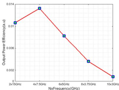
**Fig. 59. Output power efficiency of 30-GHz mmW-generation using the first five pairs of comb lines, or harmonics.**
