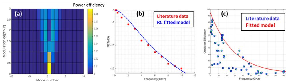
**Fig. 58. (a) Simulated efficiencies for comb line generation, using modulator parameters from [3]; (b) bandwidth of the modulator [3]; (c) microwave oscillator efficiency based on a literature study.**
