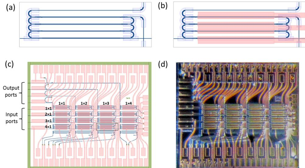
**Fig. 32. (a) Single switching element composed of three race-track micro-rings. (b) Electrodes (in red) place on the top of directional coupler for fine tuning. (c) Full layout of the chip, including the optical wiring layer (in black) and the metal wiring (in red). (d) Photograph of the fabricated chip.**
