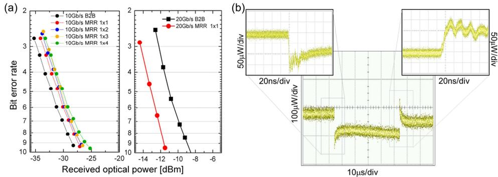
**Fig. 33. (a) Bit error rate for 10 and 20 Gbps line rates. (b) Time traces for switching time: falling time in the left-hand side inset and rising time in the right-hand side inset.**
