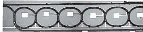
Fig. 2: Photograph of the first rings of a slow wave delay line realized with directly coupled ring resonators. The diameter of the rings is approximately 1.24 mm, corresponding to a FSR=50GHz.
