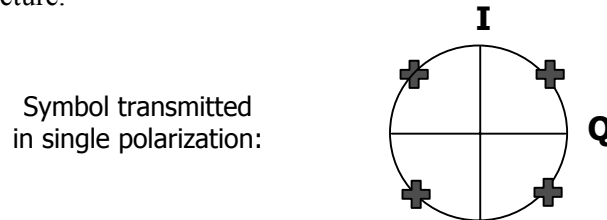
Figure 1. QPSK modulation principle (2 bits/symbol).
